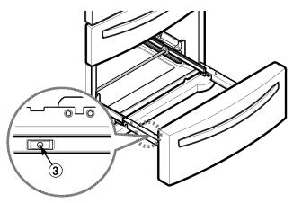
**4.** With the drawer pulled out to full extension, insert the lower basket in the rail assembly.
